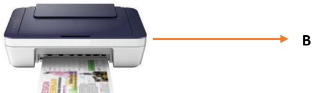
Printer is a device that accepts text and graphic output from a computer and transfers the information to paper, usually to standard size sheets of papers. There are two main types of printers. These are,
